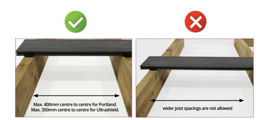
Joists must be set to a maximum of 400mm centres for Portland (350mm Ultrashield). This is to ensure stability and also to avoid warping and cracking of the deck boards.
