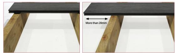
The overhang of the board should be a maximum of 20mm.
