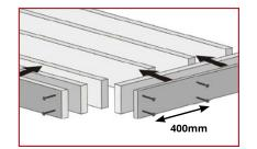
Fascia boards need to be fixed at installed on 400mm centres to prevent warping or buckling. All fascias need to use two screws 40mm away from the ends regardless of the thickness.
