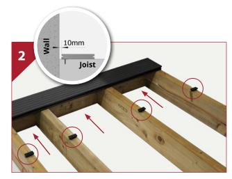
Insert a standard clip into each deck board in line with joist and screw fully but do not over tighten.
