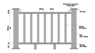
Note: Portland hand rail is only suitable for installation to a maximum of 600mm above ground level.
