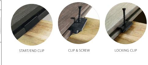
One locking clip to be installed at the centre point of each board to control even expansion and contraction along the length of the board. The locking clip has teeth on one side to catch the board.
